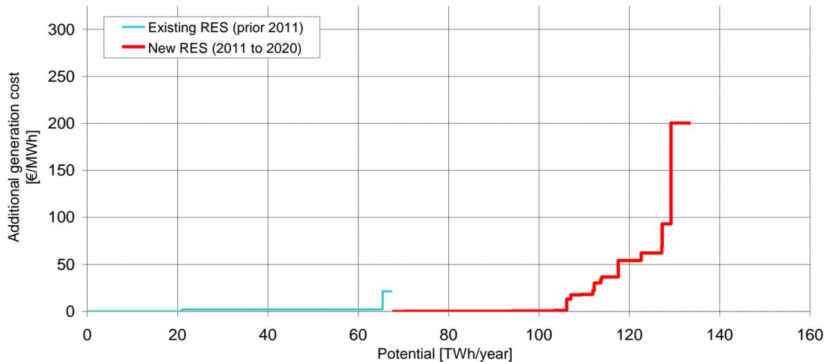
**Figure 59: Schematic dynamic cost-resource curve illustrating the feasible RES deployment up to 2020 considering dynamic aspects**
