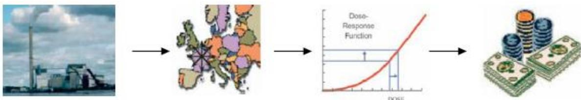
**Figure 25: Principal steps of the impact-pathway approach for estimating external costs of air pollution (Source: Bickel & Friedrich et al., 2005)**
